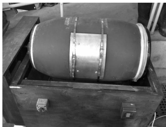
Figure 1. The tumbling barrel constructed with funds from the John Wymer Bursary.
